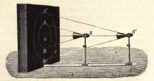
when the conical collecting mirror of the thermo-electric pile is turned towards a uniformly hot surface, the effect on the galvanometer is the same at all distances, so long at
